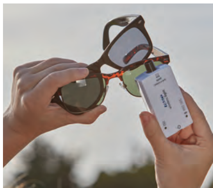
Use the ultraviolet sensor on the back side to measure the amount of UVA and UVB radiation that makes it through sunglasses.
