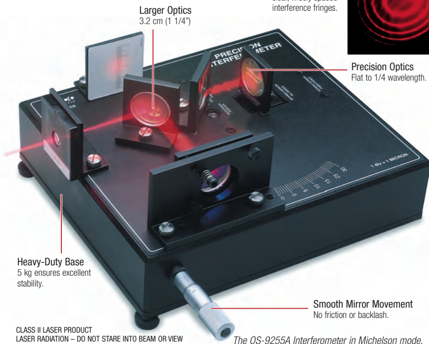
The OS-9255A Interferometer in Michelson mode.
