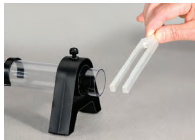
The Resonance Air Column can be used as a closed or open tube. In the closed mode, tuning forks or speakers are suitable for sound sources. In the open mode, a speaker with a signal generator is required to vary the frequency until the tube sounds a resonance.
