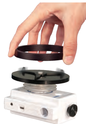
The angular speed of the disk decreases when the ring is dropped onto the spinning disk.
