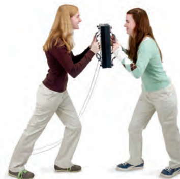
Confirm Newton's Third Law by pushing on a Force Platform using two sets of handles (available separately). Handles bolt onto the Force Platform (1-axis or 2-axis) and can be mounted on one or both sides.
