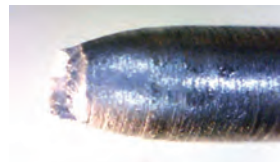
Image of broken steel tensile sample taken with the microscope.
