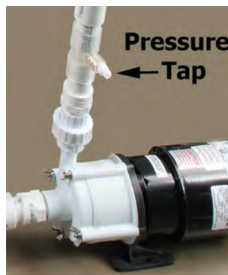
The pressure is measured just above the pump as the water velocity is varied.
