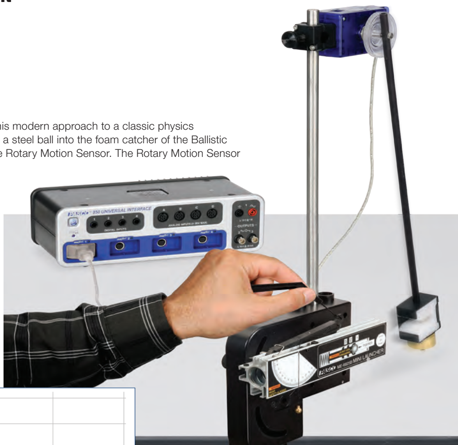
The ball is shot into a foam catcher at the end of a pendulum. The pendulum is mounted on a Rotary Motion Sensor to record the entire swing.
