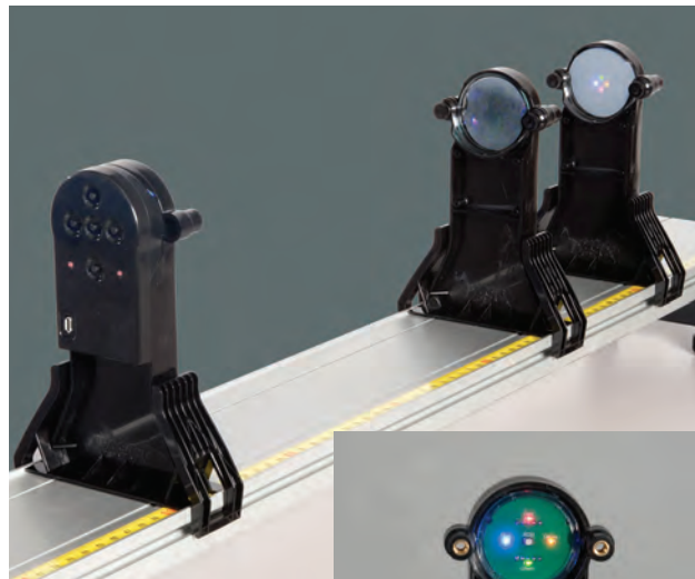
Lens holders mount to PASCO tracks.
