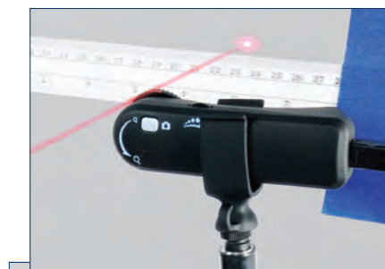
The USB Camera Microscope records the oscillation of the laser beam.
