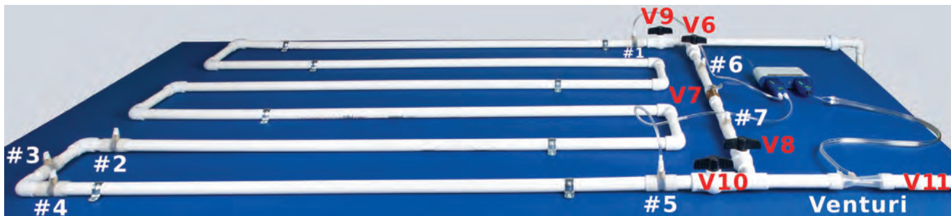
Two pumps are operated separately and then together in series and parallel.
