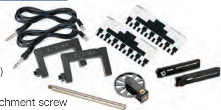
Position and velocity graphs are obtained using a Picket Fence and Photogate.
