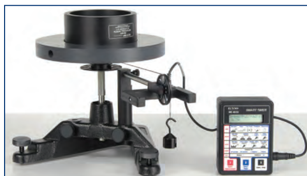
Rotary motion—In Acceleration: Linear Pulley mode; the Smart Timer measures the acceleration of the string over the Smart Pulley.
