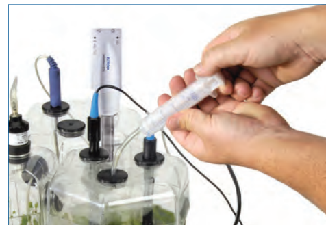
Keep the system closed during chemical testing – use the included syringe to extract water. Or inject pollutants into the system and see how the ecosystem responds.
