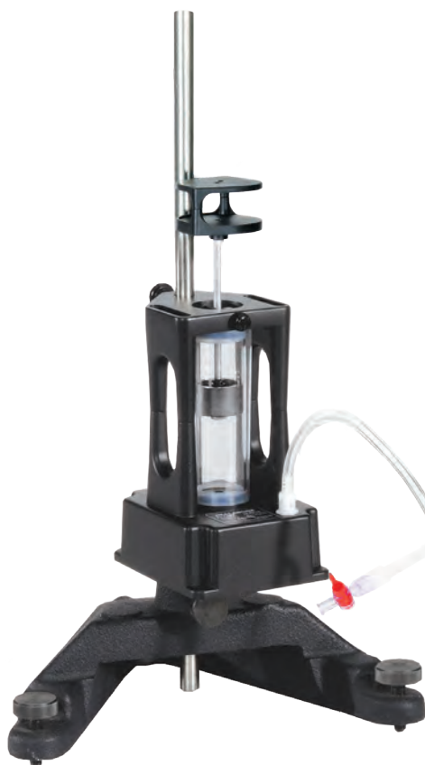
The pressure oscillates after the piston is plucked by hand.
