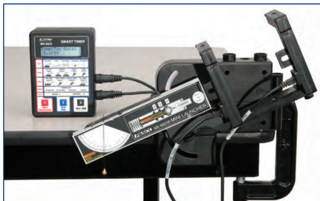
Speed of projectile—In Time: Two Gates mode; determine the speed of a ball fired by a Projectile Launcher through two photogates.
