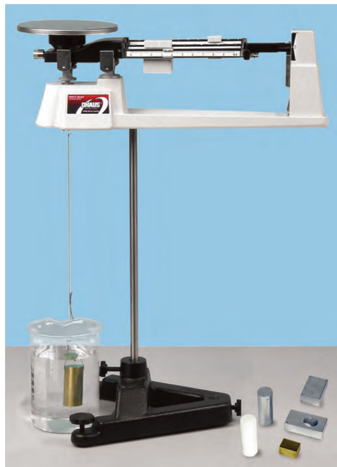
The mass and volume are measured to determine the dependence of the buoyant force on mass, volume, and density.
