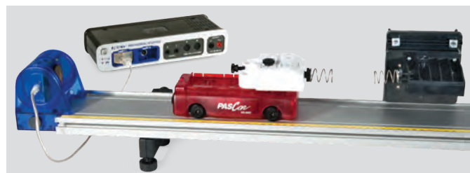
Wireless Force Acceleration Sensor (PS-3202) in cart collisions with fixed spring bumper on Force Bracket
