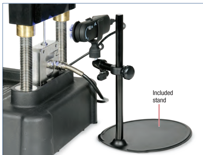
Shown in use with ME-8236 Materials Testing Machine (see page 160). As the tensile sample is being stretched, the force versus time data is graphed in sync with the movie.
