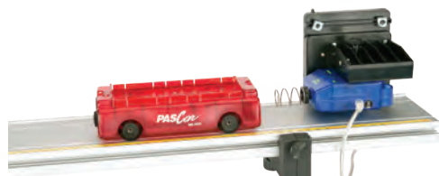
Wireless Force Acceleration Sensor (PS-3202) in cart collisions with fixed spring bumper on Force Bracket
