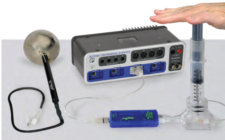
For the Ideal Gas Syringe (shown above) the Slope of the Volume vs. \frac{1}{P} graph equals nR .
